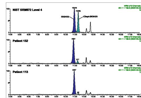
Figure 3. Chromatographic separation of 25OHD3 from the corresponding C3-epimer.
